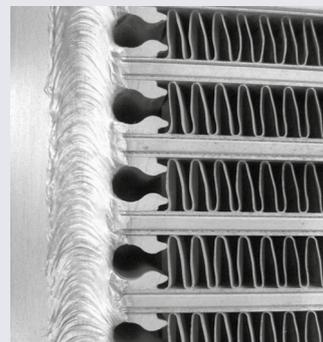
AKG-Line uses AKG hollow profiles to reduce local peak strains. This way the strength of heat exchangers is significantly increased and their service life time considerably prolonged.
