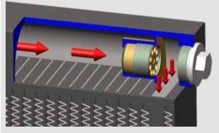
The installation of an external bypass is not necessary reducing costs and mounting space.
