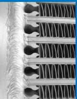
In many coolers AKG uses hollow profiles to reduce local peak strains. This way the strength of heat exchangers is significantly increased and their service life time considerably prolonged.
