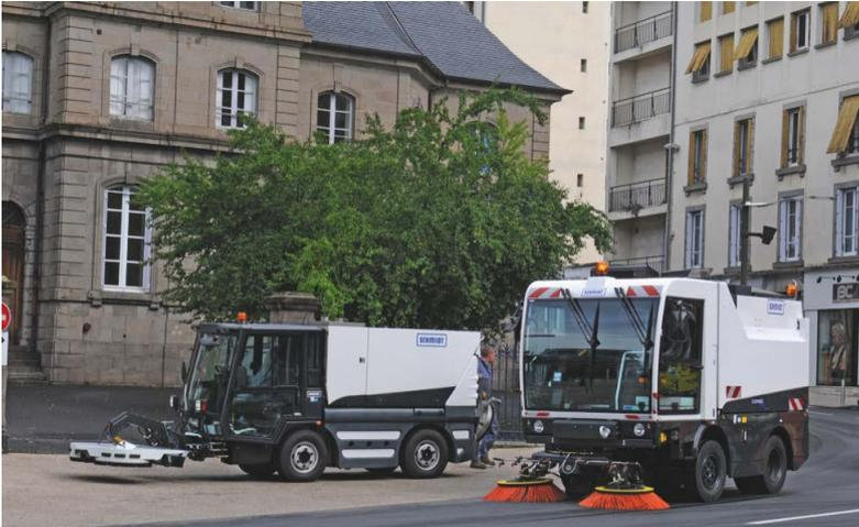
The Aebi Schmidt *Cleango 500* is a compact sweeper made by Aebi Schmidt. The *Cleango* is used for street cleaning in municipalities and industrial areas and has a disc brush system under the driver's cabin. The cooling module that is used is specially designed for cleaning vehicles to ensure optimal cooling performance.
